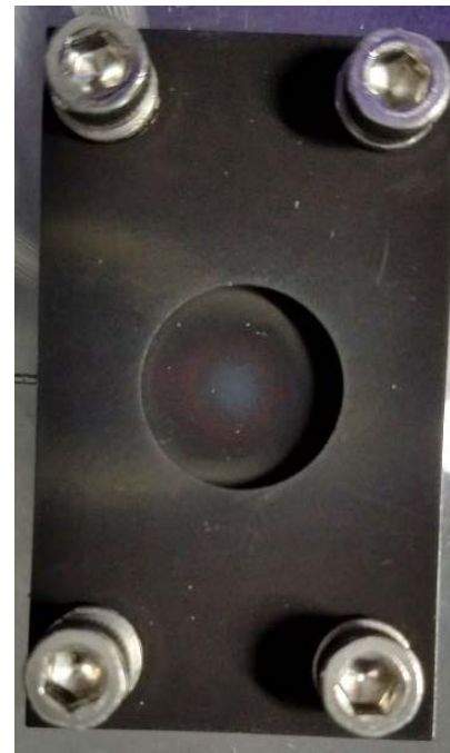
Inconel mock window coated with very high temperature (VHT) thermal paint.
